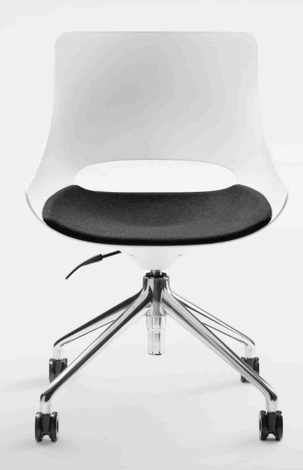
The chair shell is a complex injection moulding that was carefully developed through many iterations, from card and paper models, CNC foam and fiberglass prototypes prior to investment in tooling.
