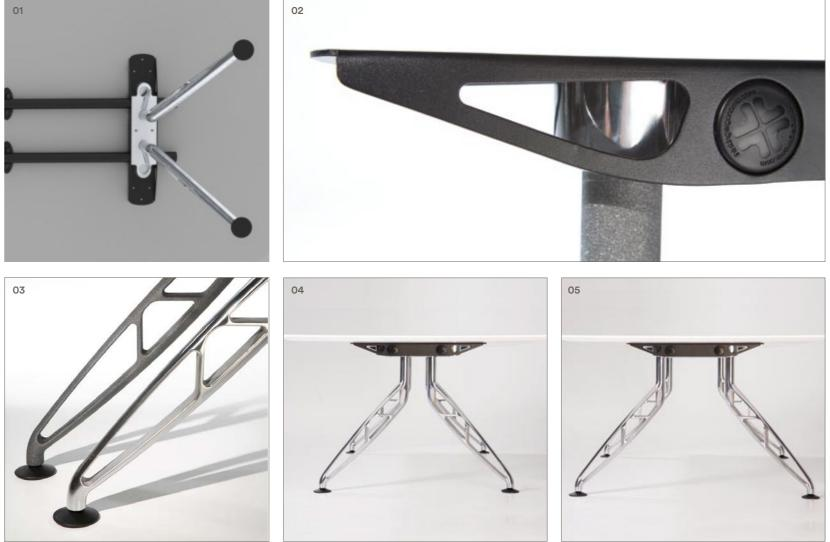
a steel threaded insert which is encased in the die cast aluminium. The steel thread provides a much stronger connection from the top horn to the leg than if the aluminium was threaded for attachment to the top horn
