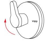
1. Mount the suction hook on the surface by applying pressure to the plastic hook.
