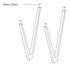
6. Remove the gliders with a flatheaded screwdriver.
