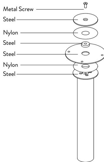
3. Screw counterclockwise to loosen and divide the turn joint.
