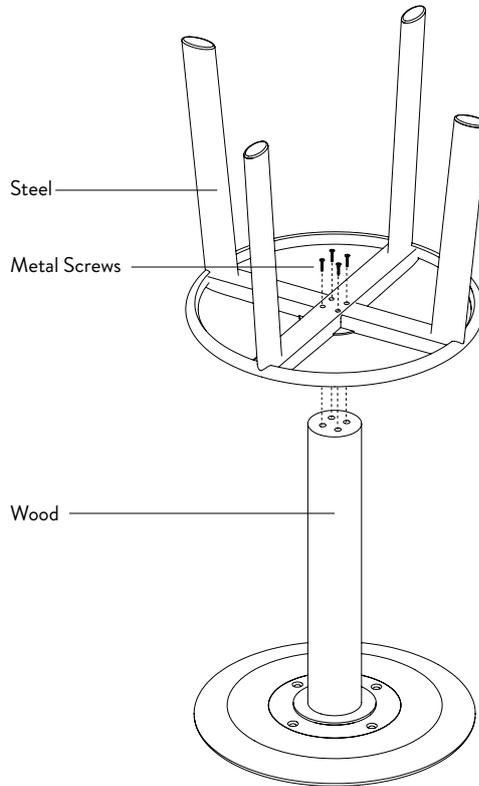
2. Screw counterclockwise to loosen the seat from the rod.
