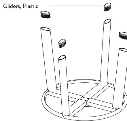
4. Remove the gliders with a flatheaded screwdriver.
